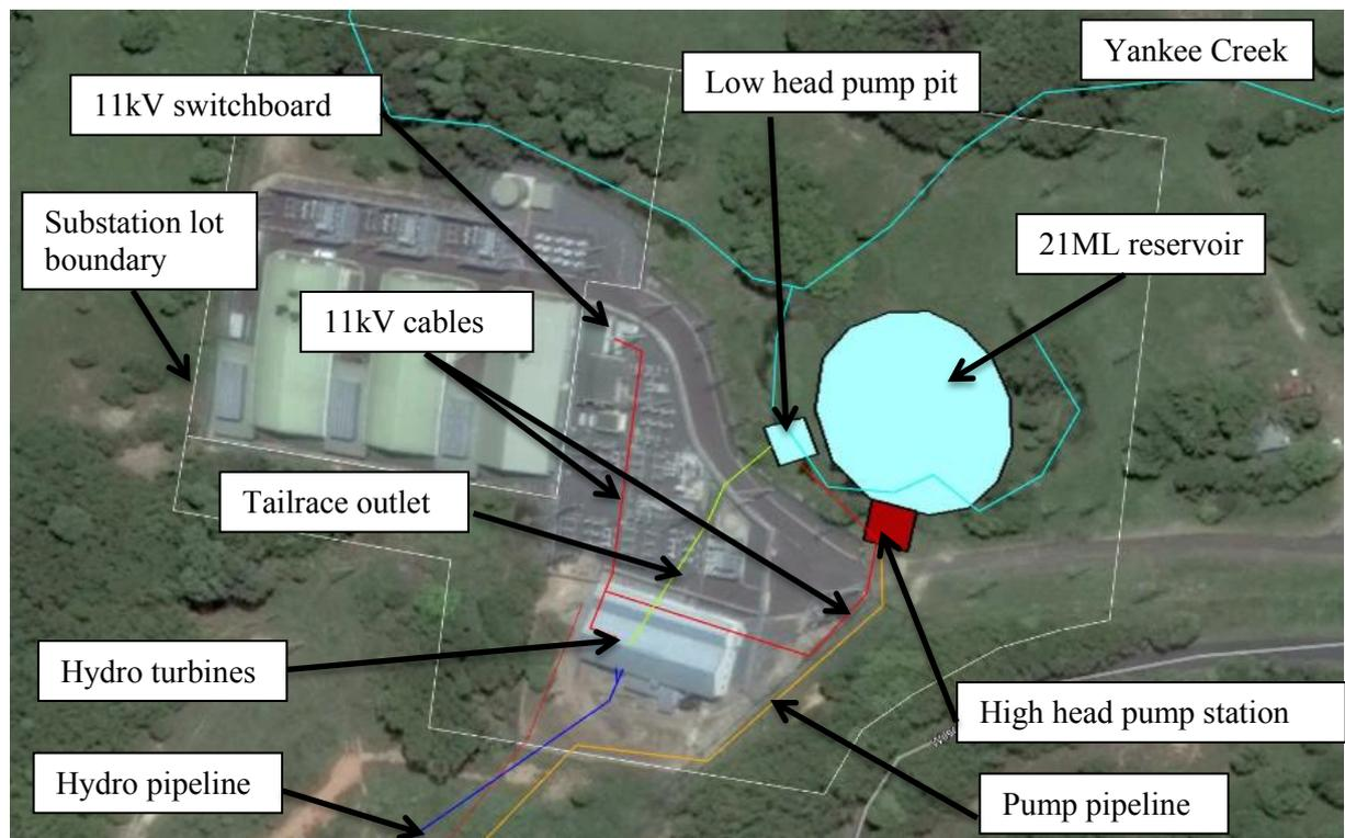
Figure 3.2: Detail at hydro/pump station
