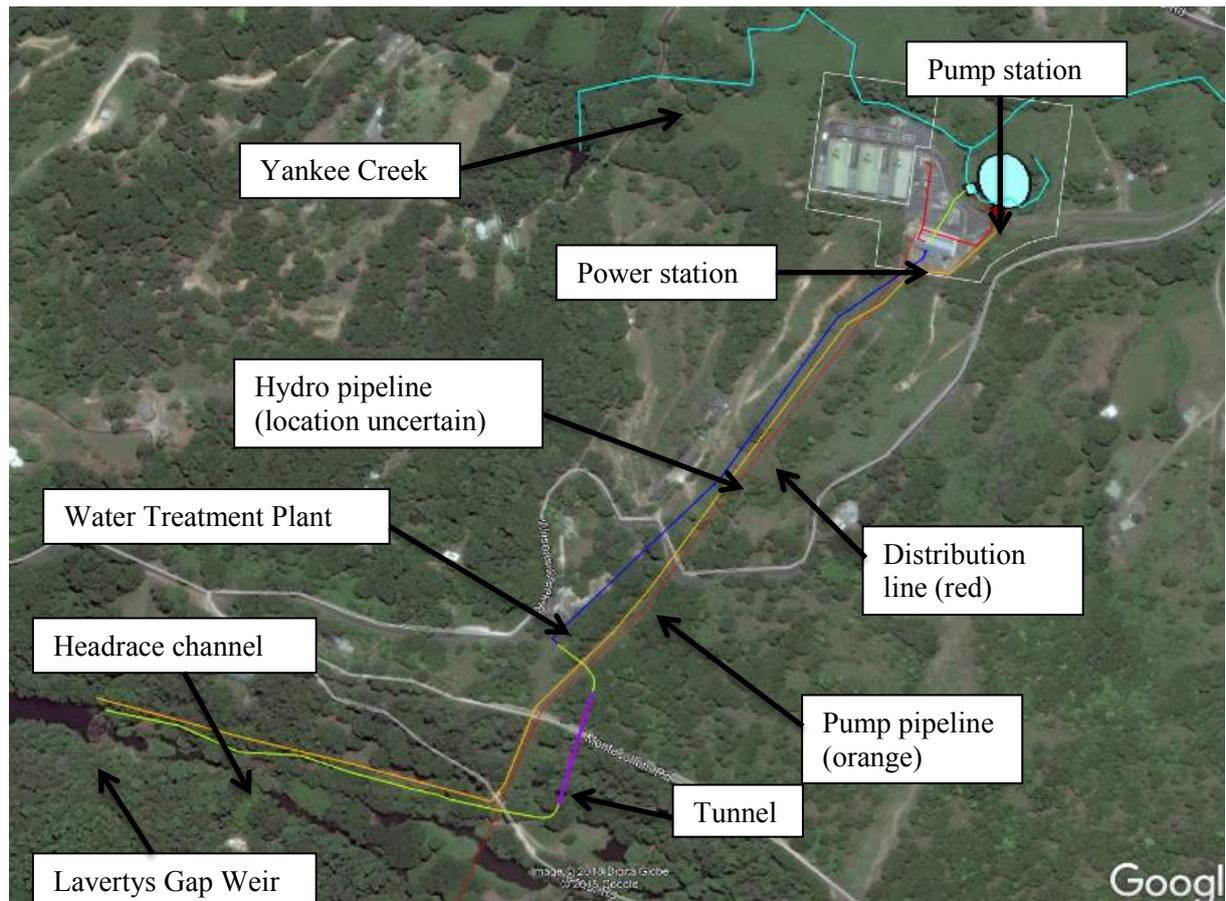
Figure 3.1: Scheme general arrangement
